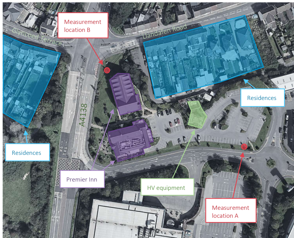
Figure 3-1 Satellite image (courtesy of Google) with measurement location, nearby noise sources, and noise-sensitive receivers highlighted
